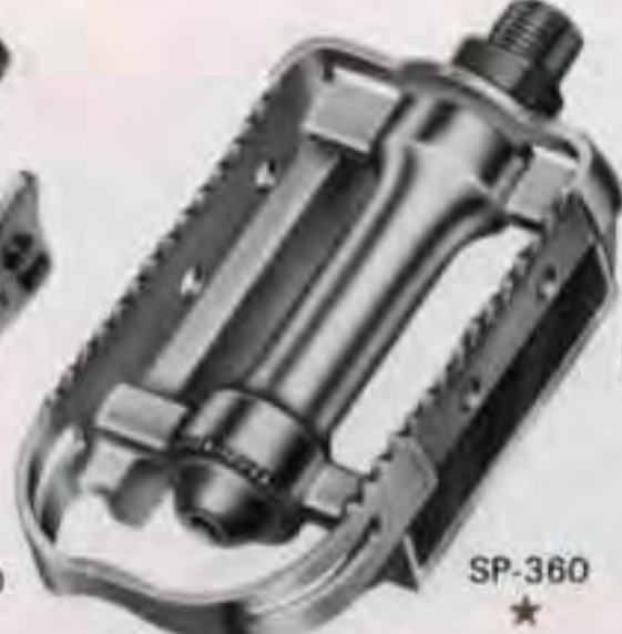
Model SP-360 SILSTAR PEDAL-360 One piece frame. Quill type. With reflector. Foot on size: 60mm(2 3/8")×105mm(4 1/8") Thread: BC 3/8"×20T M14×P1.25 Weight: 460g(16.1oz)
