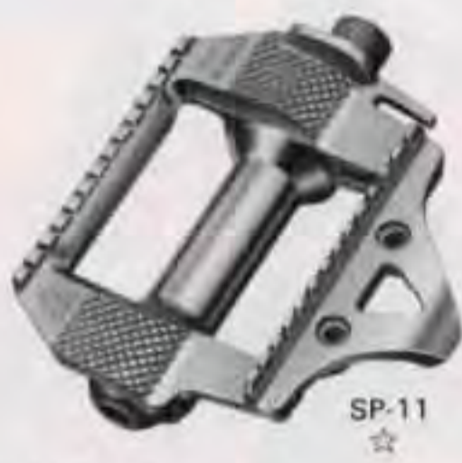
Model SP-11 SILSTAR PEDAL-11 One piece frame. Platform type. Cr-Mo steel spindle. Foot on size: 60mm(2 3/8")×88mm(3 1/2") Thread: BC 3/8"×20T or M14×P1.25 Weight: 380g(13.3oz) Toe clip, Strap and Reflector attachable.
