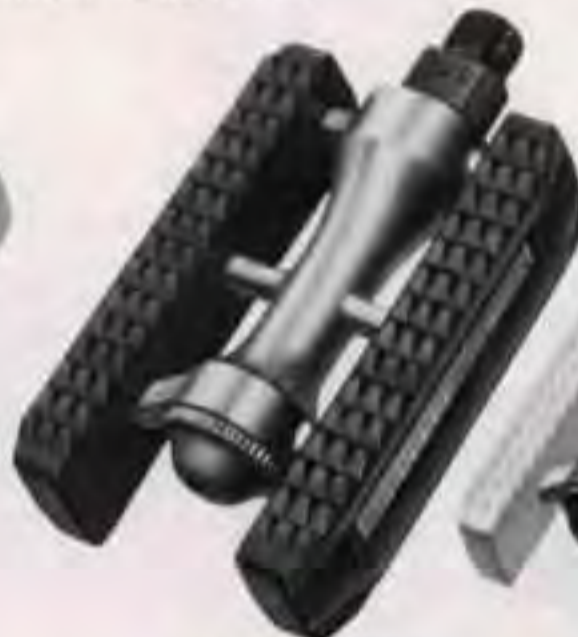
Model SP-550FW (White) SP-550FB (Black) SILSTAR PEDAL-550FB, FW One piece frame. Full rubber type. Foot on size: 65mm(2 5/8")×98mm(3 7/8") Thread: BC 3/8"×20T or M14×P1.25 Weight: 500g(17.5oz)
