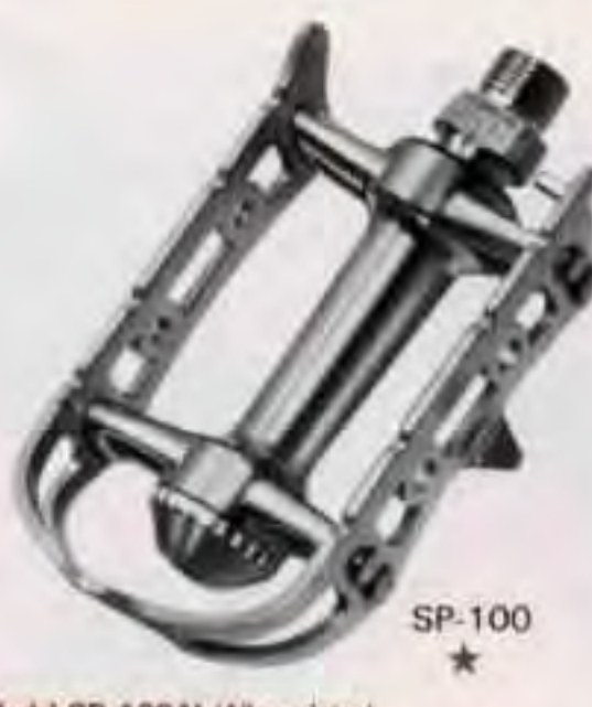
Model SP-100AL (Alloy plates) SP-100BL (Alloy plates black finish) SP-100CP (Steel plates) SILSTAR PEDAL-100AL, BL, CP Quill type. Foot on size: 61mm(2 3/8")×100mm(4") Thread: BC 3/8"×20T or M14×P1.25 Weight: 100AL, BL 345g(12.8oz) 100CP 420g(14.7oz) Toe clip, Strap and Reflector attachable.
