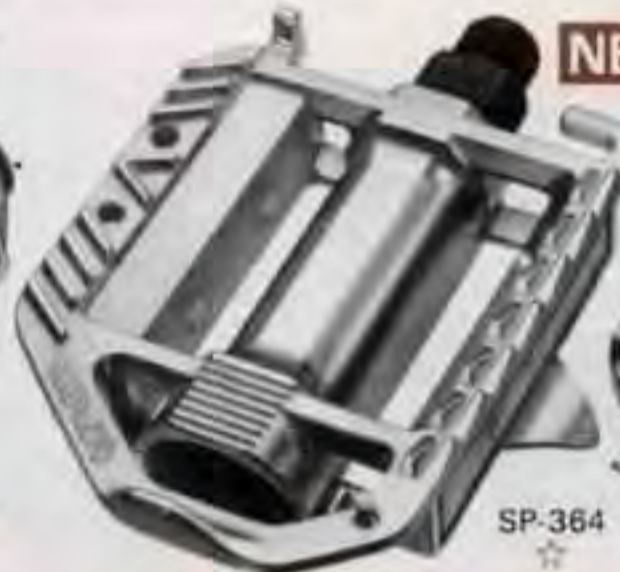
Model SP-364 SILSTAR PEDAL-364 One piece frame. Self-Balanced pedal. With Reflector. Foot on size: 75mm(3")×100mm(4") Thread: BC 3/8"×20T or M14×P1.25 Weight: 550g(19.3oz) Toe clip and Strap attachable.
