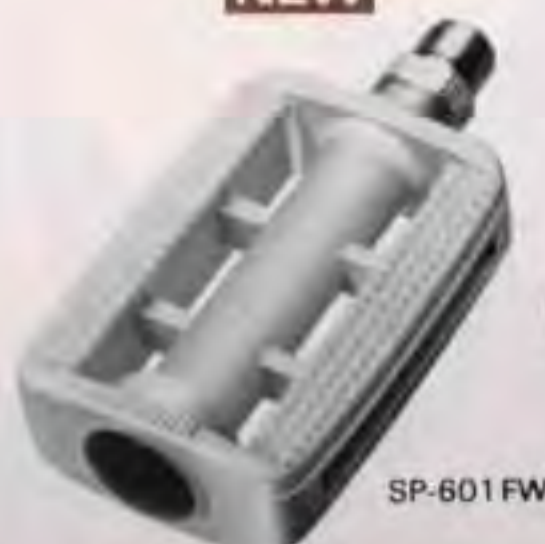
Model SP-601FW (White) SP-601FB (Black) SILSTAR PEDAL-601 Made of plastic one piece frame. For juvenile. Foot on size: 55mm(2 1/8")×92mm(3 5/8") Thread: BC 3/8"×20T Weight: 290g(10.2oz)
