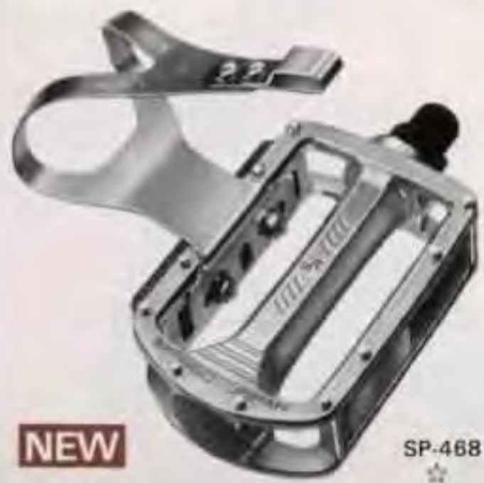
Model SP-468 SILSTAR PEDAL-468 One piece frame. With Reflector. Foot on size: 64mm(2 1/2")×95mm(3 3/4") Thread: BC 3/8"×20T or UNF 1/2"×20T Weight: 410g(14.4oz) AC-30, AC-40 Toe clip attachable.
