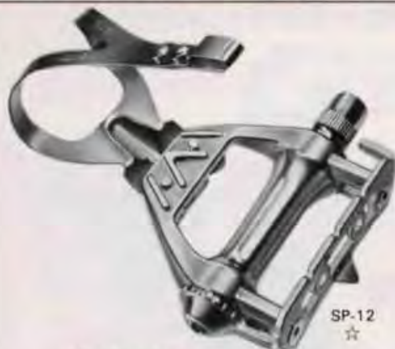
Model SP-12 SILSTAR PEDAL-12 Aerodynamic type. Cr-Mo steel spindle. Foot on size: 75mm(3")×70mm(2 3/4") Thread: BC 3/8"×20T or M14×P1.25 Weight: 370g(13oz) AC-45 Toe clip attachable.
