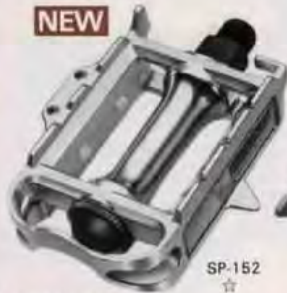
Model SP-152 SILSTAR PEDAL-152 One piece frame. Quill type, with Reflector. Foot on size: 61mm(2 3/8")×100mm(4") Thread: BC 3/8"×20T or M14×P1.25 Weight: 410g(14.4oz) Toe clip and Strap attachable.
