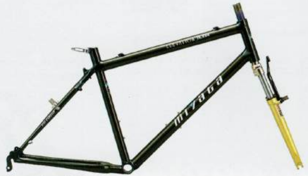
Elevation 10000 • Full Carbon Fiber APA Bonded Frame • Super Oversized Tubing • Front Suspension Fork
