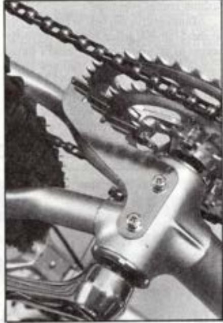
Miyata worked so hard on the bottom bracket lug and were so proud of it, they added an anti-chain suck plate to keep the area from getting bugged up. Nice touch.
