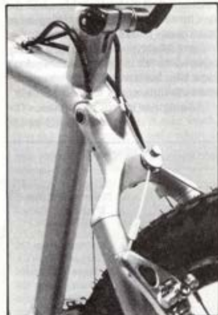
A whole lot of work went into this piece, and a whole lot of weight came out. It was clean and stiff, but the kinks in the rear brake cable made for less than optimal brake effectiveness in the rear.
